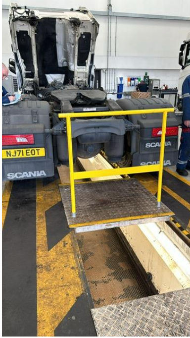
Photo 6: When you need to carry out inspection tasks or minor repairs use the pit bridge placed under the vehicle and fitted with a handrail.
